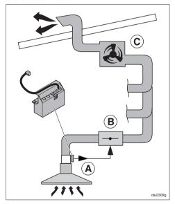
The potential free contact on the DSM 400 (a) can, for example, be used in a cooker hood with an external motor ...EXT, which is connected to a central ducting system.
